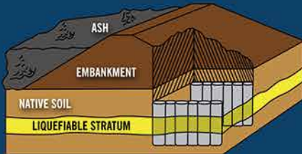
JET GROUTING FOR LIQUEFACTION MITIGATION
