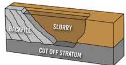
SLURRY TRENCH GROUNDWATER CUT-OFF
