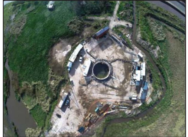
► Aerial view of Shaft #3 showing perimeter ground freezing system.
