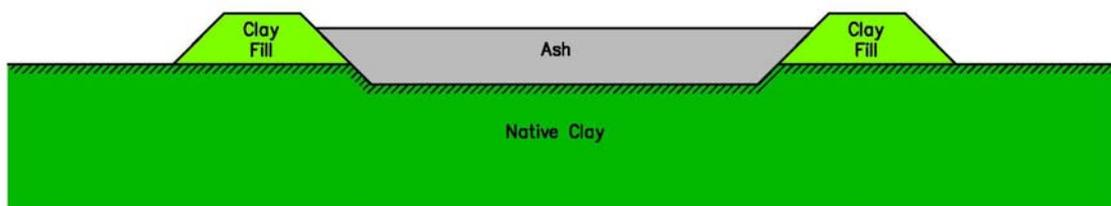
Figure 1: Generalized cross-section through Pond 2. (Not to scale)
