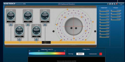
Figure 8: Instrumentation screen shot of CP No. 2 temperature and pressure acquisition
