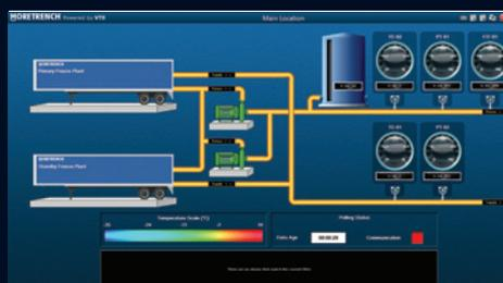
Figure 7: Instrumentation screen shot of the coolant distribution manifold system data
