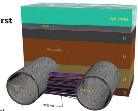
**Above: Figure 1 - Tunnels Below the Channel; Right: Figure 2 - Cross Passage arrangement**
