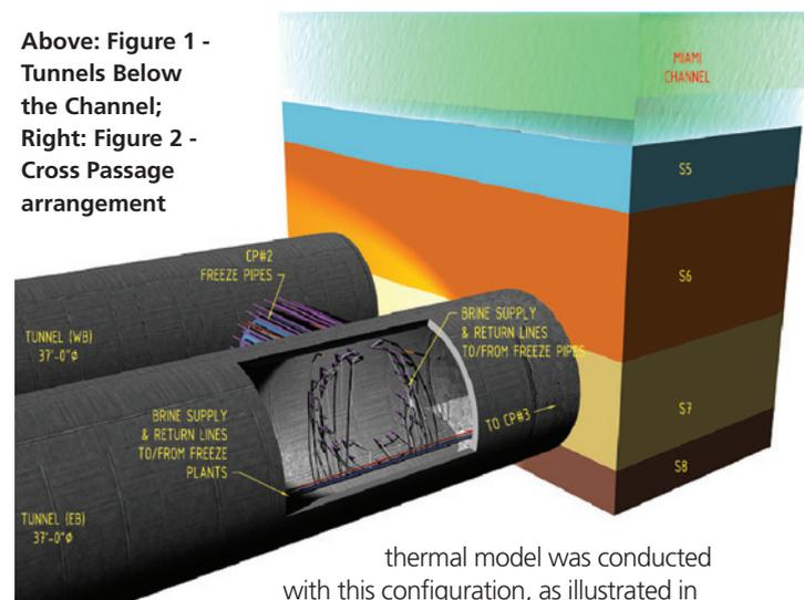
thermal model was conducted with this configuration, as illustrated in Figure 3. The two rings of freeze pipes were drilled and installed from the eastbound tunnel. These pipes had an immediate contact with the tunnel lining on the exterior of the tunnel and a frozen seal could be easily attained. The situation was somewhat different westbound end of the cross passages.
